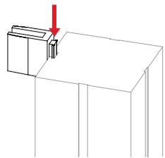
Slide connector on back of A10 clamp into groove of extrusion.
